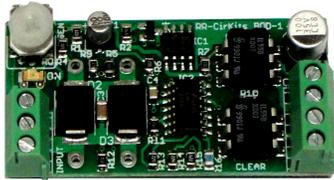
**Sensing** The BOD-1 uses the voltage drop across 3 Amp Schottky diodes for detection. Normal detection levels are 1ma. for use with 10K wheel sets. Sensitivity may be decreased to 15ma. with the on board potentiometer for situations requiring less sensitivity. To further reduce sensitivity place a resistor across either one of the diodes. Using Schottky diodes
